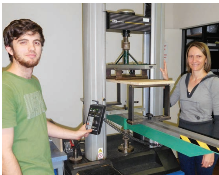
EWPA laboratory manager Suzie Steiger monitors an Instron machine used for testing the bending strength and stiffness of plywood, particleboard and MDF samples at the Eagle Farm laboratory in Brisbane while new recruit Troy Edwards adjusts calculations on the machine.
